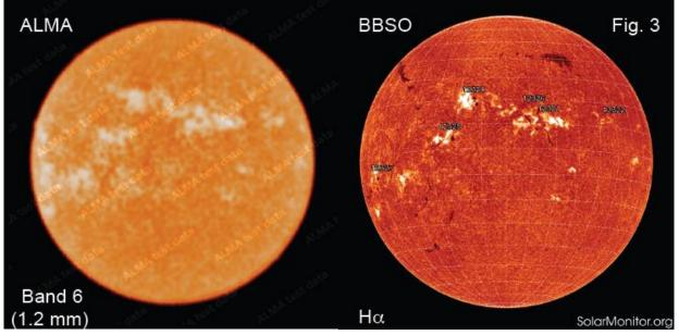
Resolution: Band 3 (3 mm): 60" Band 6 (1.2 mm): 24" Band 7 (0.9mm): 18" Band 9 (0.4mm): 9"
